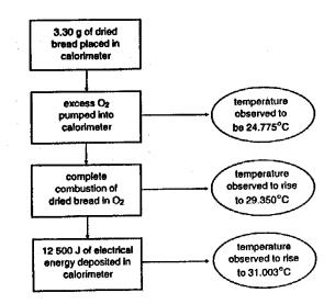
(a) Calculate the calibration factor of the calorimeter plus contents.
